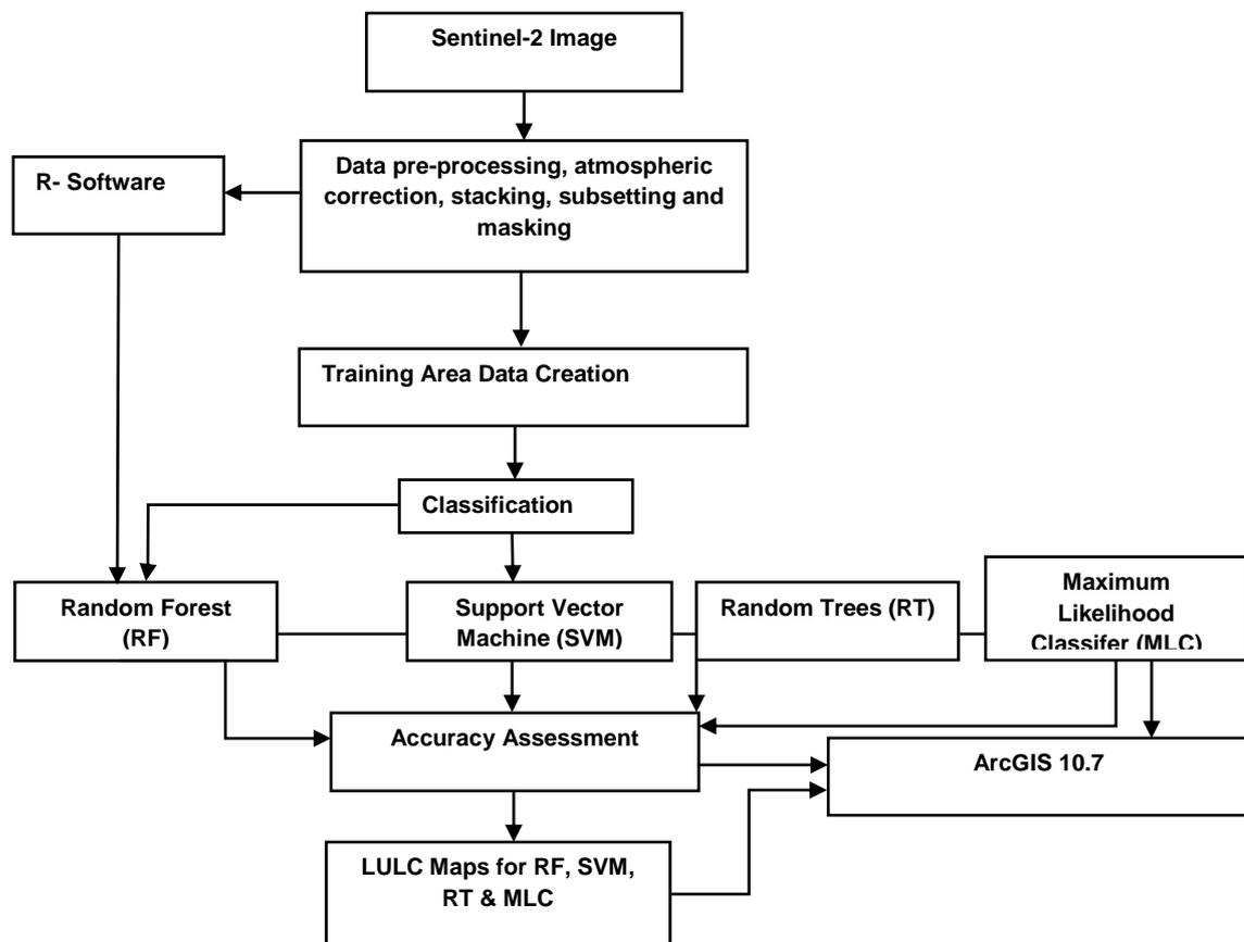
Figure 3 Procedural workflow from pre-processing data to comparison of classification results.
