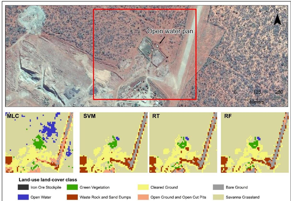
Figure 5 Maximum Likelihood Classifier (MLC) identifying open water classes where there were none, in contrast to the right classification made by the three machine learning algorithms: Support Vector Machine (SVM), Random Tree (RT), and Random Forest (RF).
