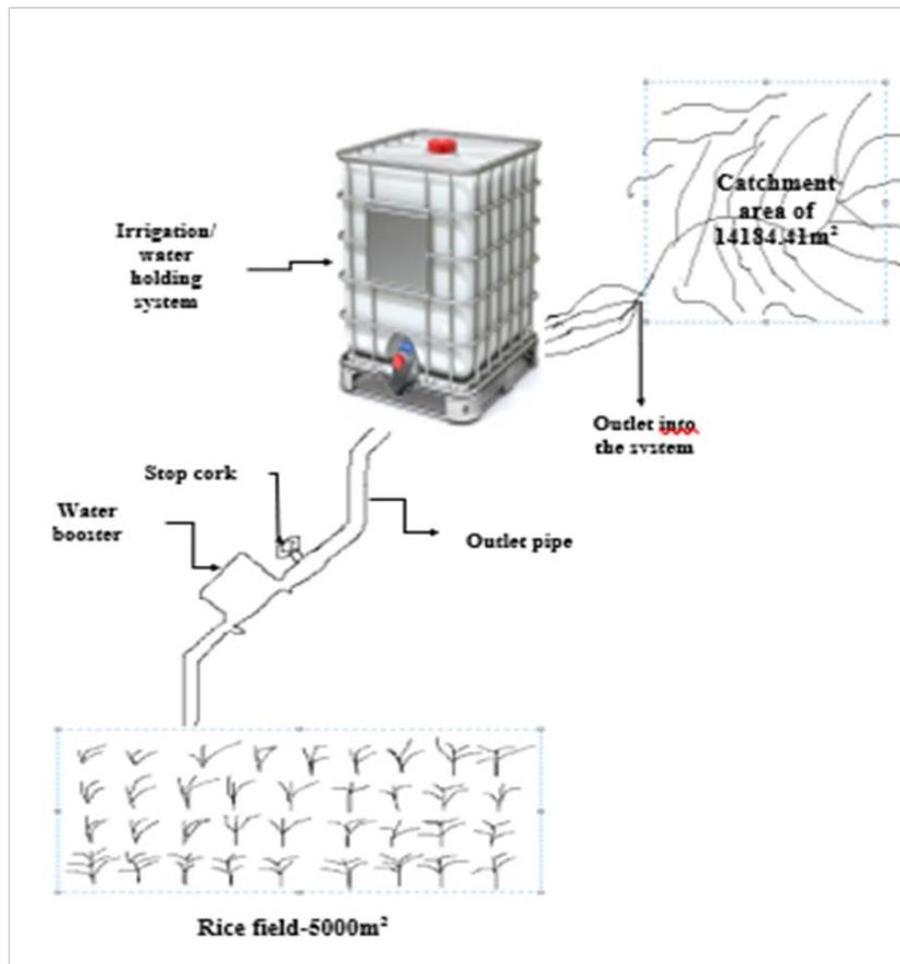
Figure 6: Supplementary Irrigation Scheme (Source: Author's Construct)
